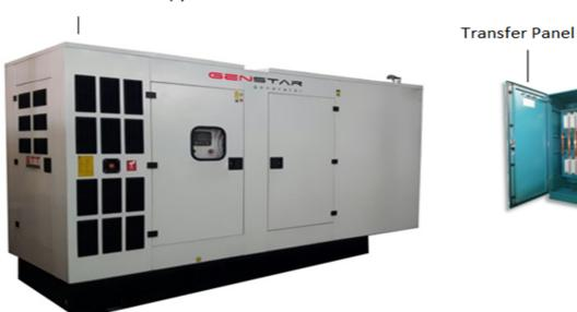
**5.2- Chassis:** All equipment of the generator is mounted on the steel chassis, inside of it the fuel tank is available. Diesel suction and return hoses, fuel filler cap, fuel level indicator float, lifting holes located on the generator chassis (frame). The fuel tank is designed to feed to the generator at least eight hours of continuous operation. External fuel tank is provided for the generators above 1100 kVA power. Engine and alternator are mounted on chassis with anti- vibration mounts .
